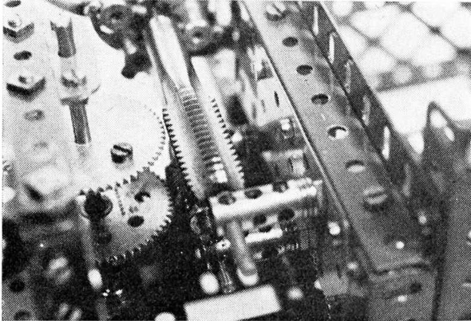
A view of the main frame without the cutting carriage and main bearing assembly. The horizontal feed for the carriage appears at the near end of the frame.
