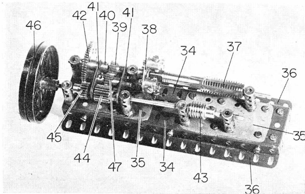
Top, a “working” Meccano model in the true sense of the word is this Gear-cutting Machine, designed and built by the author. It will produce real gears from a variety of materials.
