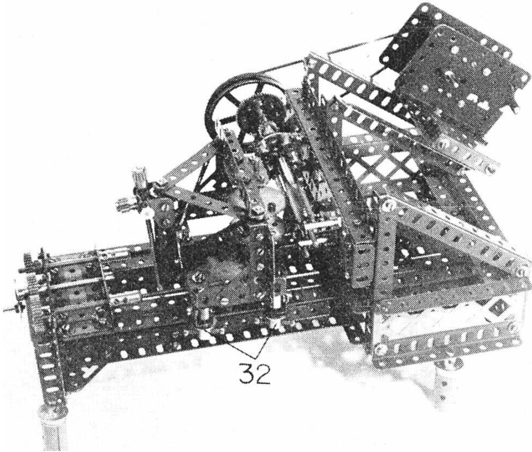
A detailed view of gear-cutting in operation. As the lower Meccano Gear Wheel makes contact with the Worm, when fed in horizontally (from left to right), the Tap begins cutting the upper disc. The Worm and Tap drive are coupled in a 1:(1):1 ratio.
