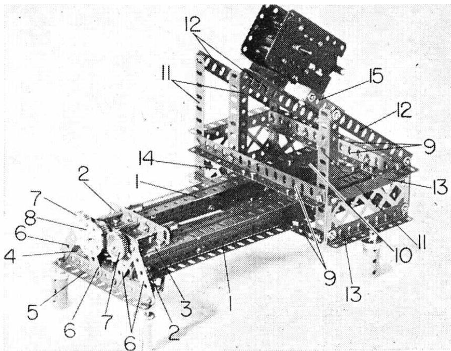
The cutting carriage as it appears removed from the Machine. In the right foreground is a P.V.C. disc prepared ready for cutting and a completed gear cut from brass.
